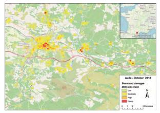
Figure 3 - Simulated losses for the 2018 Aude event aggregated on a 250m grid.
