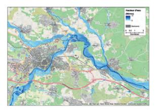
Flooding estimated by the Floodos model for the Aude River flood (2018).
